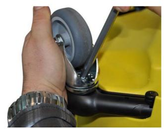
→ Use an Allen key with ball head to loosen the screws.
