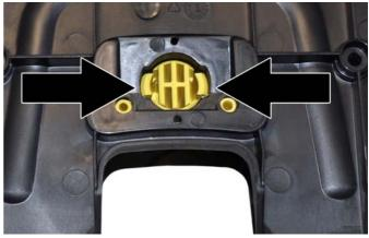
→ Press the locking tabs together with pliers and, at the same time pull the key out of the housing toward the top.
