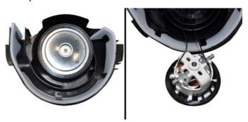
→ Remove the suction turbine from the turbine holder.
