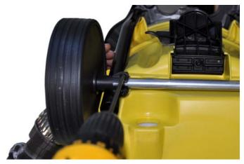
→ Unscrew the screws on both axle bearings.
