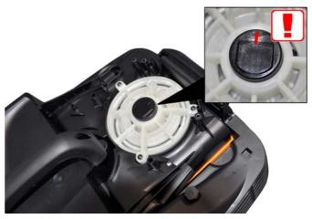
→ Observe the alignment of the slide cap (arrow) during installation.
