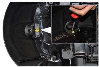
→ Press the locking tabs together with pliers and, at the same time pull the key out of the housing toward the top.
